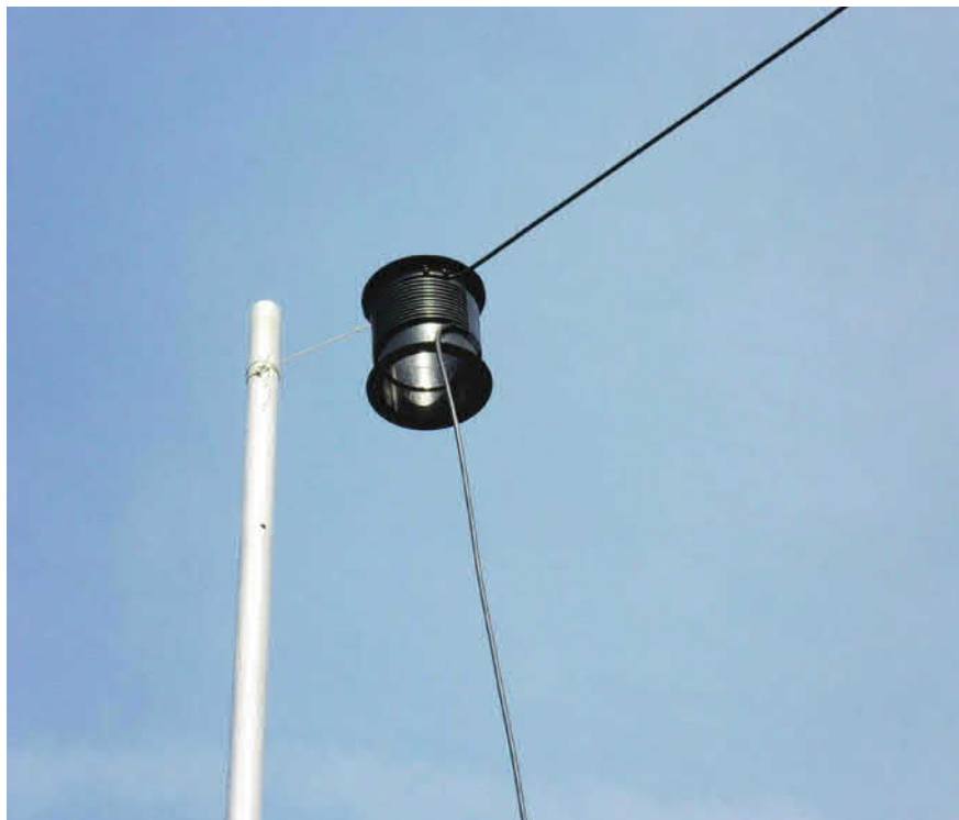
PHOTO 1: The CFR dipole's RF choke formed from 12 turns of coax cable.
