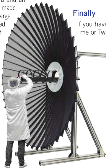
The unfurlable reflector antenna from Oxford Space Systems. Photo courtesy OSS.
