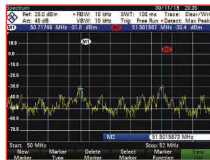
FIGURE 3: Class D audio amplifier frequency spectrum 50-52MHz.
