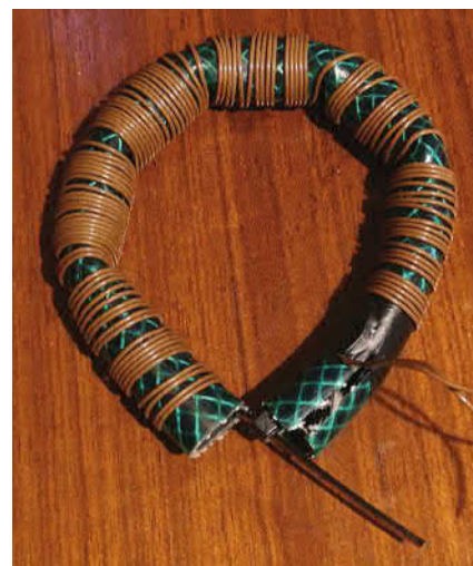
Experimental Rogowski coil on a piece of garden hose.
