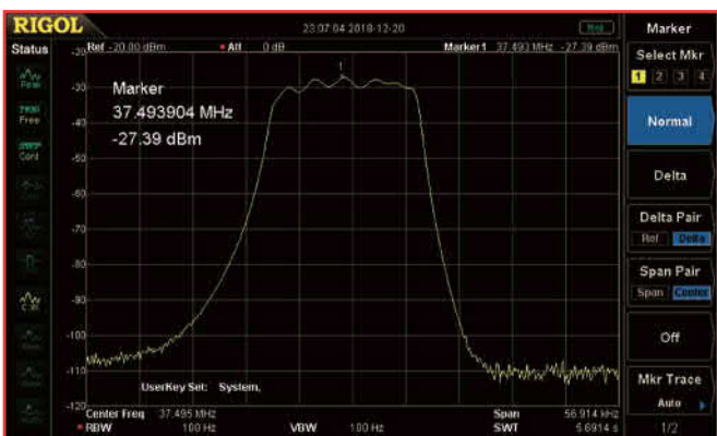
FIGURE 7: 15kHz filter narrow scan frequency response. Centre frequency 37.492092MHz, span 50.502kHz.
